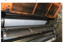
Ink is rolled onto an offset cylinder or blanket - which is transferring the ink to the paper
