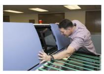
A laser will flash text on the chemical coated aluminum plate in the chamber - burning the chemical on the plate.
