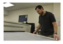
Chemical that is not heat-set is washed away in a bath. The final plate is coming out of the bath.
